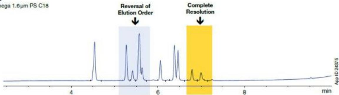
When developing methods for the analysis of highly lipophilic molecules like these, we recommend evaluating both Luna Omega 1.6 μm C18 and Luna Omega 1.6 μm PS C18, two potential solutions for this type of separation challenge.
