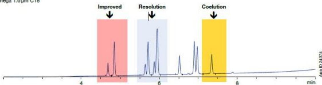
However, sometimes a brute-force approach is not always the only way to solve a problem, and evaluating phases with slightly different selectivity is an essential part of the method development process. In **Figure 3**, you can see the same separation performed using the Luna Omega 1.6  $\mu\text{m}$  PS C18, which contains a proprietary, positively charged functional group on the surface in addition to the C18 bonding. Under the exact same conditions, you
