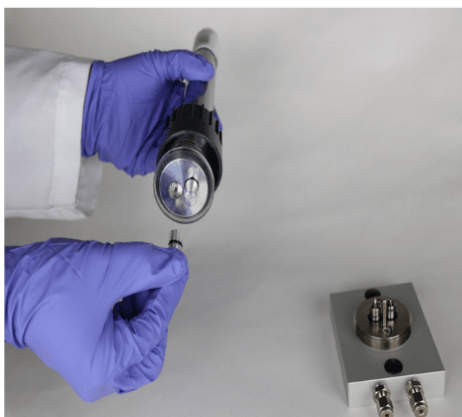
Step- 1: Remove endplugs from the cartridge style filter
